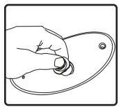
3. Remove motion sensor lens. 4. Place narrow lens into pod cover. Make sure lens is flush with outside of pod cover. Align the flat side of the lens w/ the flat side of the pod cover.
